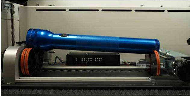
Incorrect Setup: The flashlight is not horizontal. Raise the right side of the flashlight by turning the jack screw.
