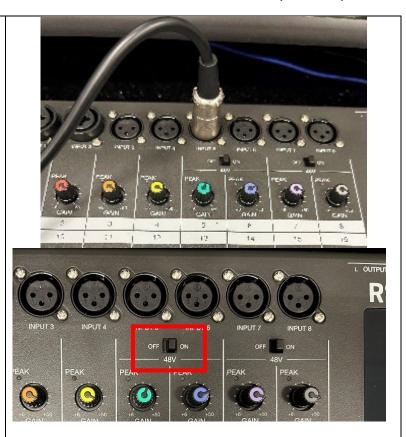
For the wireless microphones, plug the receiver to input 1 or 2 and turn on one, or both microphones.
